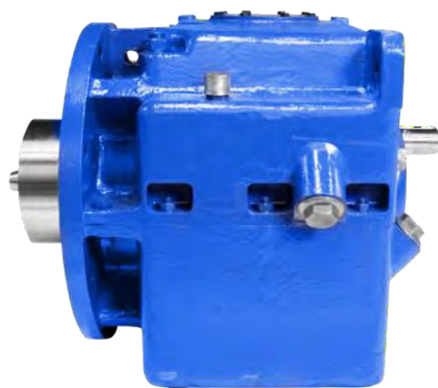
David Brown gear box after refurbishment
