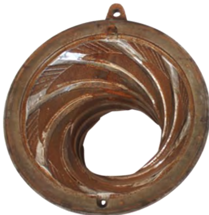
Lining for Simo® grinder before refurbishment
