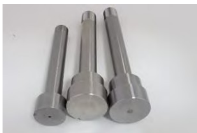
Stay bolt for drive hub, partnumber 0120-87H ✓, 0120-212H ✓, 0120-236H ✓
