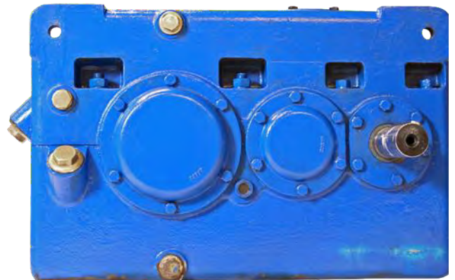
David Brown gear box after refurbishment
