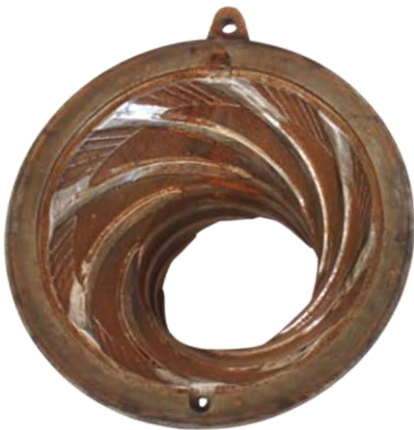
Lining for Simo® grinder before refurbishment
