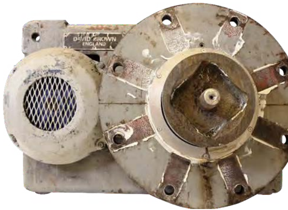
David Brown gear box before refurbishment
